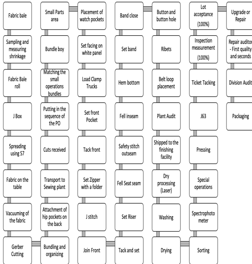
Fig. 1: Process Flow Chart of Denim Manufacturing (S7 is a spreading machine, J-Stitch is a sewing machine creating the J-shaped seam around the zipper, and J63 is a laser guided quality control machine)
