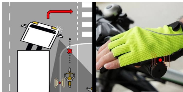
Figure 1: The cyclist is warned of a right-turning truck by a vibration signal
